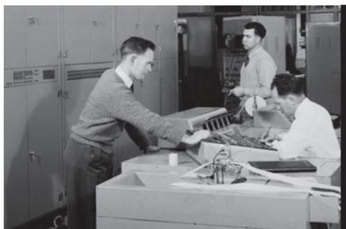
A new magnetic disc was installed replacing the magnetic drum used in Sydney. It arrived in Melbourne with the Mk1 without magnetic surface and several weeks were spent investigating a way of spraying a rotating disc with magnetic paint so that the surface was free from occlusions. The resultant magnetic disc gave excellent service. The new disc had a 1024 word capacity per side. The second side was not utilised until 1962 following extensive transistorised additions to the original circuitry.
