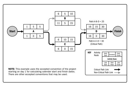
Figure 6-18. Example of Critical Path Method
