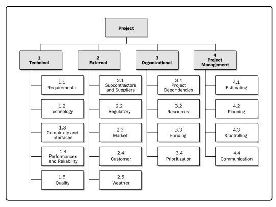
Figure 11-4. Example of a Risk Breakdown Structure (RBS)
