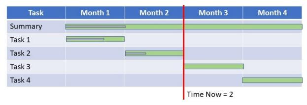
This bar chart shows both the plan (green bars) and progress (grey bars). The progress update shows 75% of Task 1 work is complete and 25% of Task 2's work; in aggregate one month's worth of progress has been achieved.
