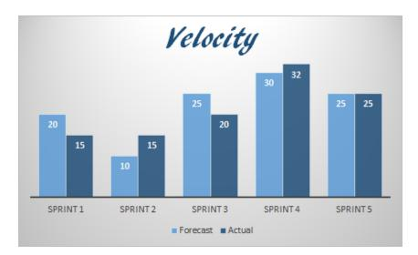
Using the velocity data, it is possible to divide the remaining backlog with the updated average velocity to determine the number of sprints needed to complete a project. Based on this estimate, if the average duration of a sprint is known (plus the number of available sprint teams), the time needed to complete the remaining work of the project can be assessed.
