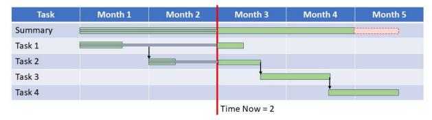
These two updating options are supported by most scheduling tools; the retained logic option shows a 4-week delay, the progress override option a 3-week delay. Neither option is right, or wrong, which is best to use depends on the circumstances and is controlled by the scheduler<sup>6</sup>.
