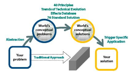
TRIZ (sometimes TIPS) is a problem-solving, analysis and forecasting tool derived from the study of patterns of invention in the global patent literature. It includes a practical methodology, tool sets, a knowledge base, and model-based technology for generating innovative solutions for problem solving<sup>10</sup>.
